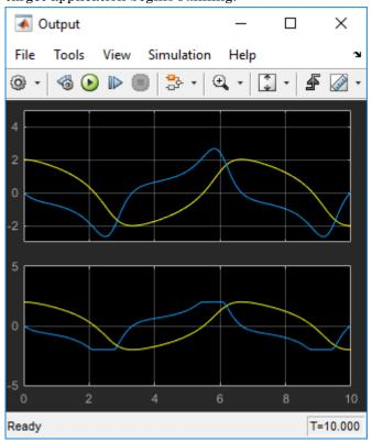
After building the model and displaying messages in the Diagnostic Viewer, the target application begins running.
