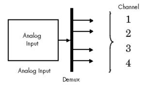
Do not specify more channels than you actually use in your block diagram. Specifying unused channels results in additional overhead for the processor with A/D or D/A conversions. In this case, for example, even though some channels are not used in the block diagram, these channels are still converted.
