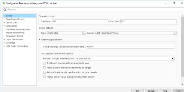
6 Leave the parameter **Treat each discrete rate as a separate task** cleared. (For models with blocks that have different sample times, select this parameter.)
