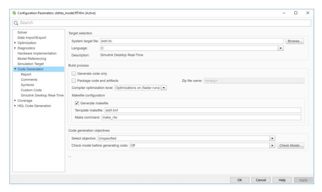
Do not set **Default parameter behavior** to Inlined on the **Signals and Parameters** node under **Optimization**. Inlining parameters is for custom targets when you want to reduce the amount of RAM or ROM with embedded systems. Also, if you select inlining parameters, you disable the parameter tuning feature. Do not inline parameters because PCs have more memory than embedded systems.
